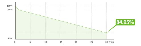
Solarspace P-type dual-glass modules Linear power output guarantee
