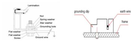
2.Ground using a grounding clamp, as shown below, containing a sliding contact, base and turning tapping screw or 8-32 bolt and hex nut. The grounding clip can hold bare copper wire in the range of 10-12 AWG.
